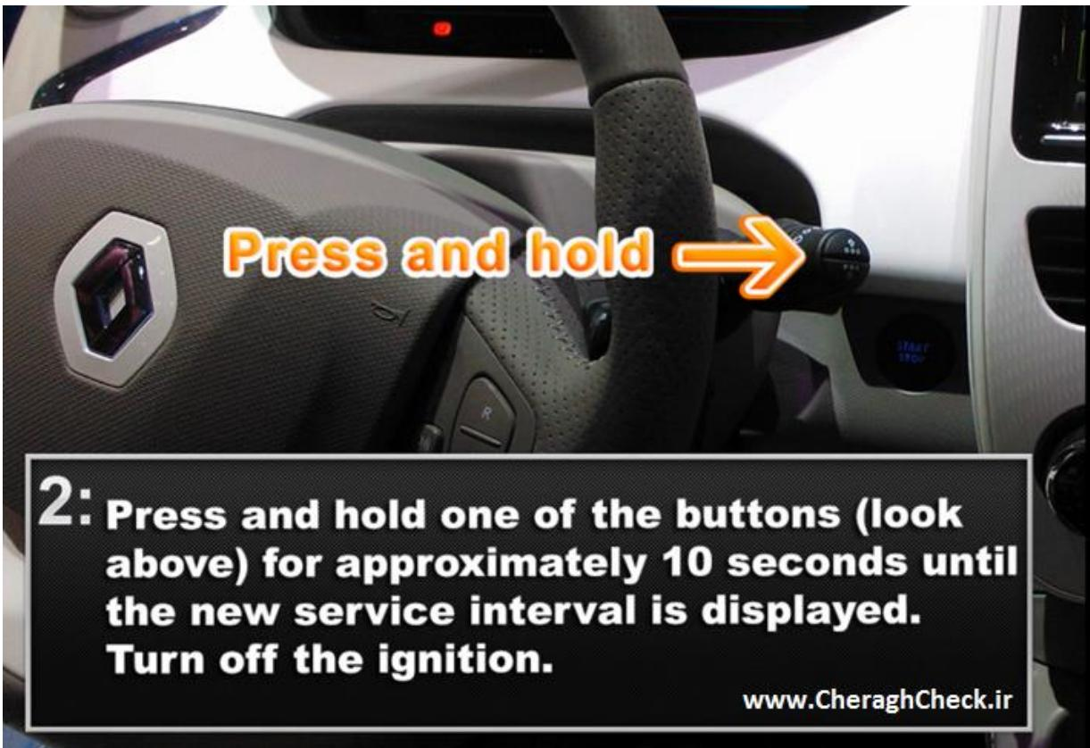
**2: Press and hold one of the buttons (look above) for approximately 10 seconds until the new service interval is displayed.**
