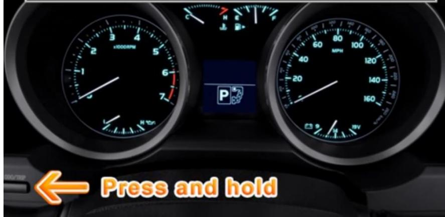
**3: The display shows "000000" for 1 second before it goes out and shows "TRIP A". The service light goes off. Release the button. Done!**
